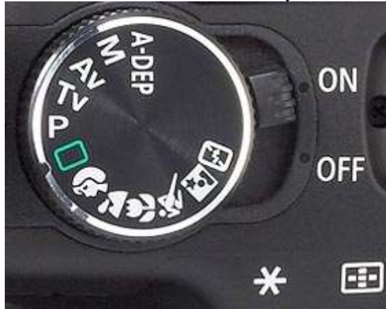
Mode dial on the Rebel XT. Above the fully automatic mode is the creative zone, below it is the basic zone.
